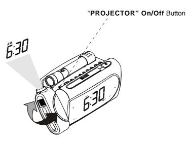
4.) If the image appears to be upside down on your wall, or upside down on the ceiling when you are lying in bed, set the **ROTATE IMAGE** switch to its alternate position.
